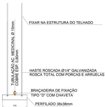
**DETALHE SUPORTE S3 PONTOS COM AR COMPRIMIDO MEDICINAL**
